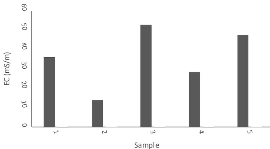
Figure 4: Electrical conductivity of soil samples measured and presented as milil Siemens per cm of dry soil.
