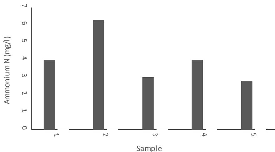
Figure 6: Ammonium N readings of soil samples presented as milligrams per litre of dry weight soil.
